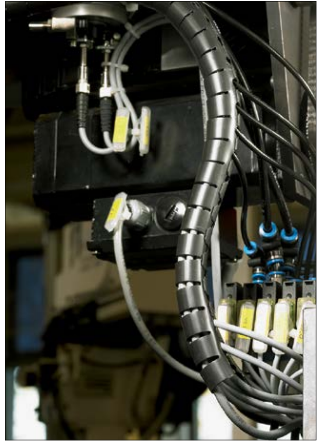
Cables can be branched off at any point for better, more flexible protection.
