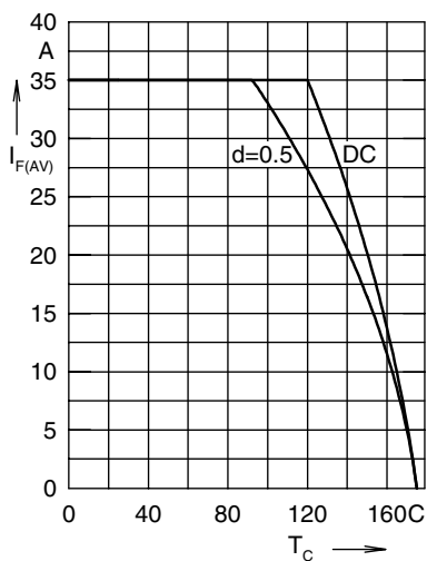
Fig. 4 Avg: forward current I_{F(AV)} vs: case temperature T_C
