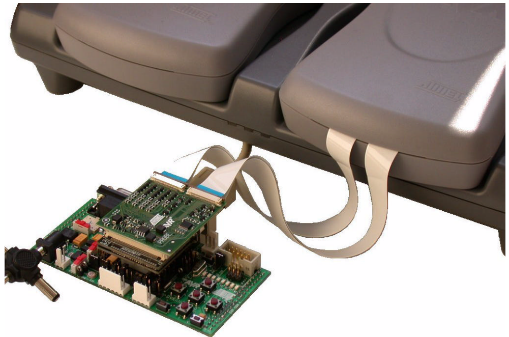
Figure 3-46 . Connecting AVR ICE 50 for Debugging
