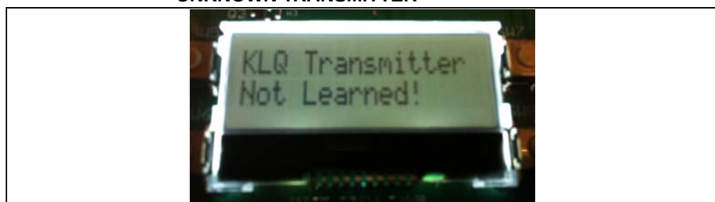
FIGURE 2-3: ERROR MESSAGE OF RECEIVING PACKET FROM UNKNOWN TRANSMITTER
