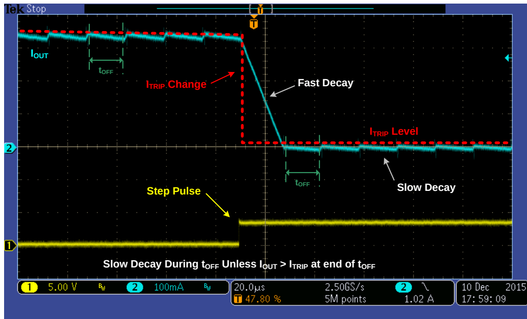
Figure 6: MP6500 Automatic Decay during Step Transition
