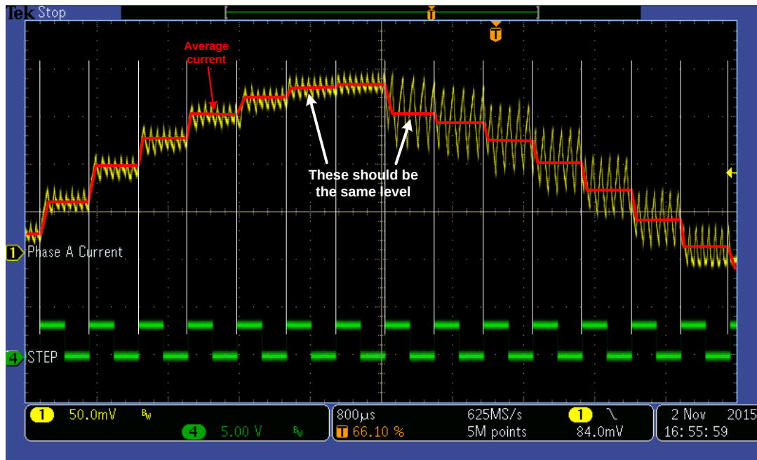
Figure 4: Conventional Current Regulation Waveform
