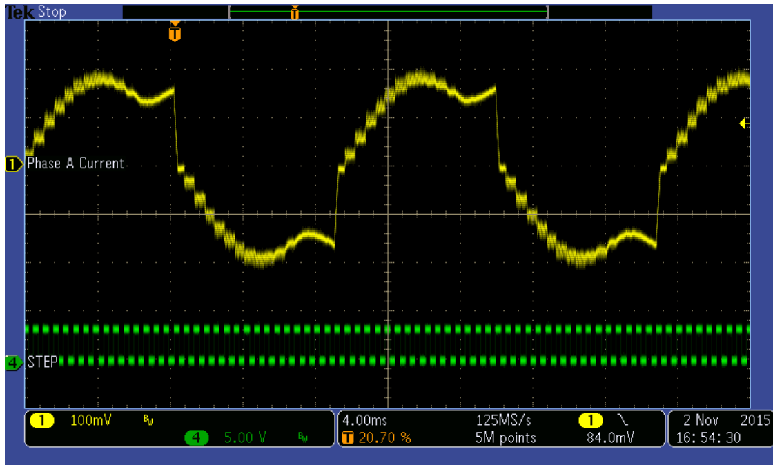
Figure 3: Current Distortion in Slow Decay Mode
