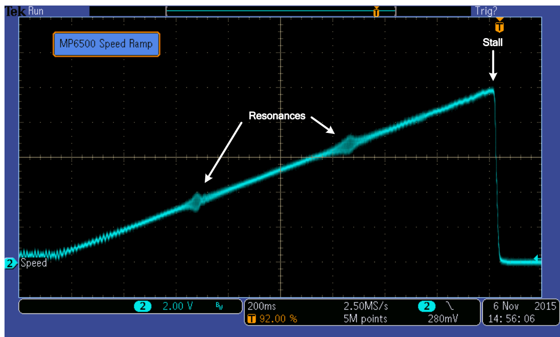
Figure 15: MP6500 Speed Ramp
