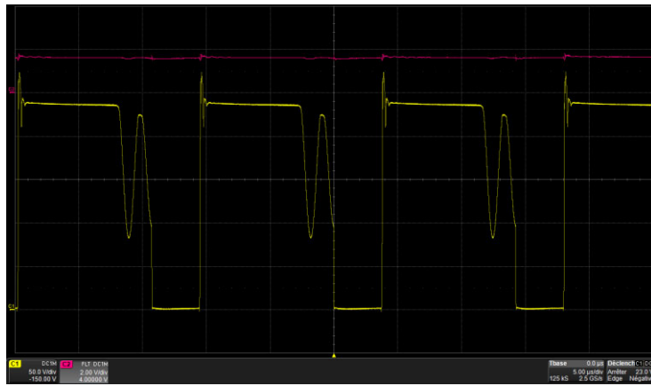
Figure 6. 2 nd Valley Operation @ 35 W / 115 V rms
