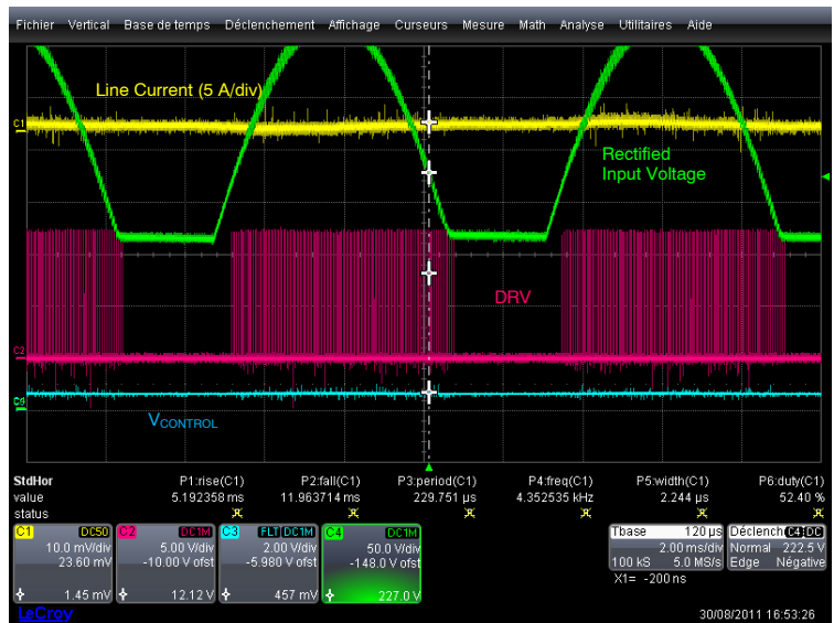
Figure 9. The Circuit Skips Cycle Near the Line Zero Crossing (265 V, 25% Load)
