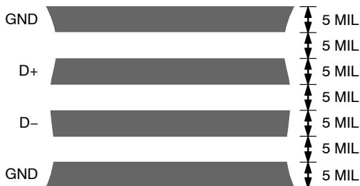
Figure 22. Typical Arrangement of Signal Tracks
