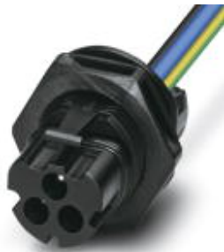
PRC device connector, black, 3-pos., 690 V (IEC 61984), 35 A, crimp connection, 6.0 mm 2 with 150 mm cable length, cut smooth at the end
