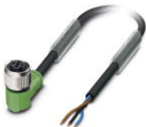
Sensor/Actuator cable, 3-position, PUR halogen-free, black-gray RAL 7021, free cable end, on Socket angled M12 SPEEDCON, A-coded, Cable length: 3 m
