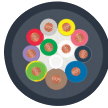
Cable cross section
