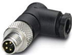
Connector, 4-position, Plug angled M8, A-coded, Solder connection, knurl material: Nickel-plated brass, external cable diameter 3.5 mm ... 5 mm
