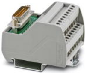
VARIOFACE module, with screw connection and D-Subminiature pin strip, for mounting on NS 35 rails, with LED, 15-pos.
