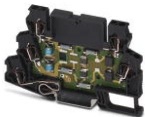
Spring cage modular terminal block with integrated surge protection, for assembly on NS 35/7.5, voltage U_N 24 V DC, terminal width: 6.2 mm, cover width: 2.2 mm
