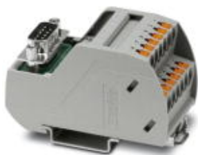
VARIOFACE module, with push-in connection and D-SUB miniature pin strip, for mounting on NS 35 rails, with LED, 9-pos.
