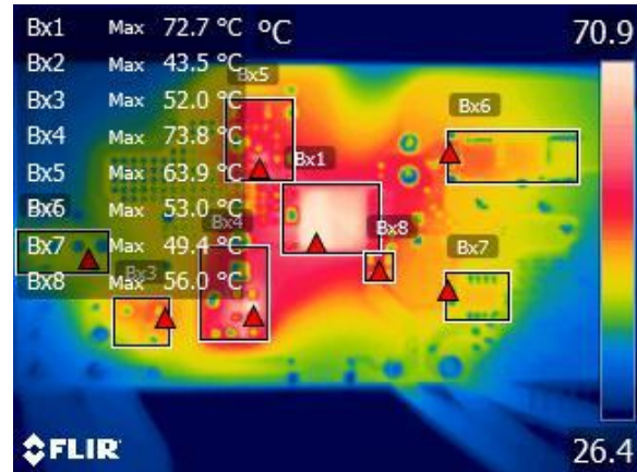
Figure 50 – Bottom Components, Ambient = 27 °C. Bx1: InnoSwitch3-Pro = 72.7 °C. Bx2: Bridge Diodes, PCB = 43.5 °C. Bx3: Thermistor, PCB = 52.0 °C. Bx4: Primary Snubber = 73.8 °C. Bx5: Auxiliary Circuit = 63.9 °C. Bx6: SR FET = 53.0 °C. Bx7: Pass FET = 49.4 °C. Bx8: Current Sense Resistor = 56.0 °C.
