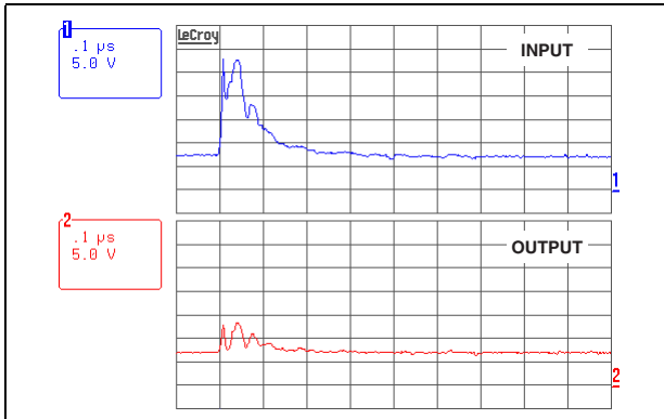
Figure 3. ESD response to IEC 61000-4-2 (+15 kV air discharge) on one input (V in ) and on one output (V out )
