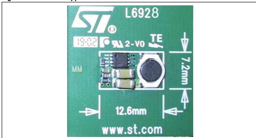
Figure 1. Minimum application board size
