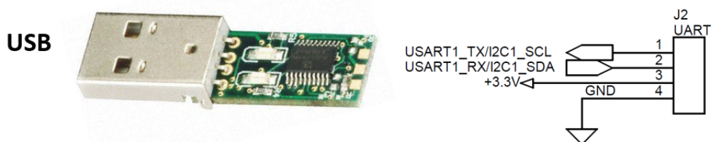
Figure 9. UART TX/RX (3v3 level)
