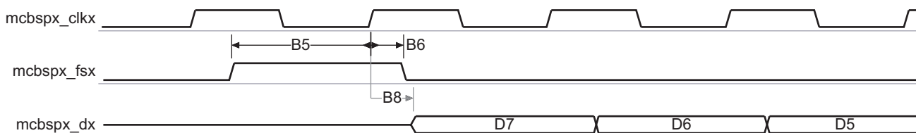
Figure 6-40. McBSP Rising Edge Transmit Timing in Slave Mode
