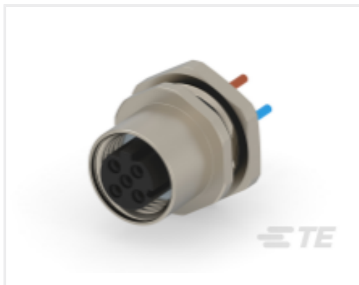
TE Part #T4171310503-001 M12,FRONT MOUNTING,FEMALE,D, 3P,0.2M WIRE
