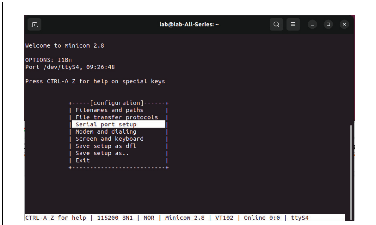
FIGURE 5-13: MINICOM SERIAL PORT SETUP
