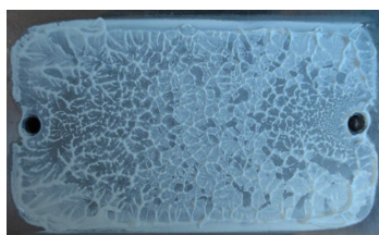
Figure 5-2. Grease on the Heat Sink After Removing the Module
