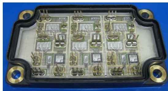
Fig. 5 Picture of the open Microsemi power module
