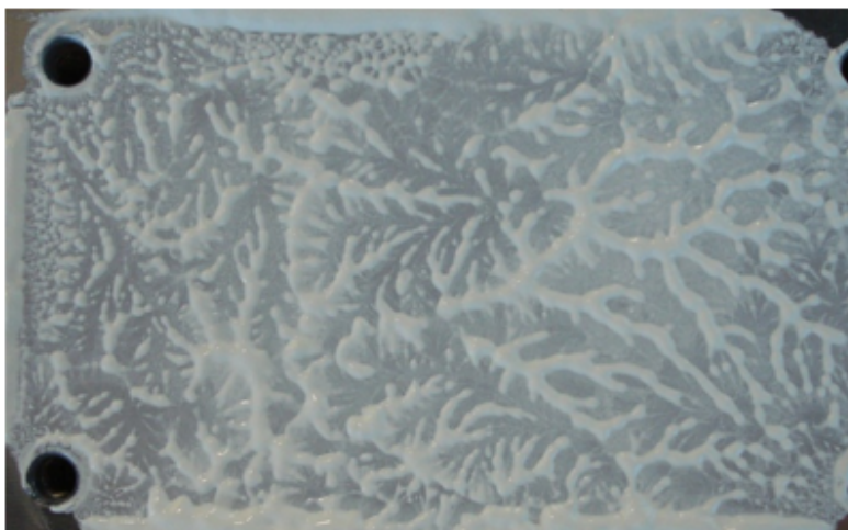
Figure 2 • Grease on the heat sink after removing the module
