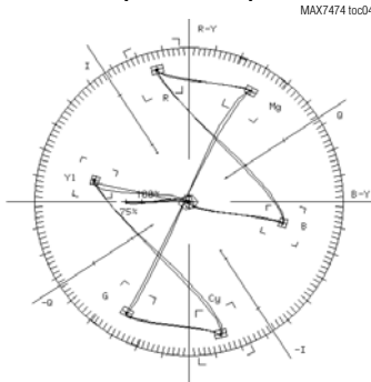
75% COLOR BAR VECTOR DIAGRAM (300m CABLE)
