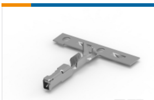
TE Part #2098762-5 Contact,female, 0.64, 20-22, CuNiSi, Sn
